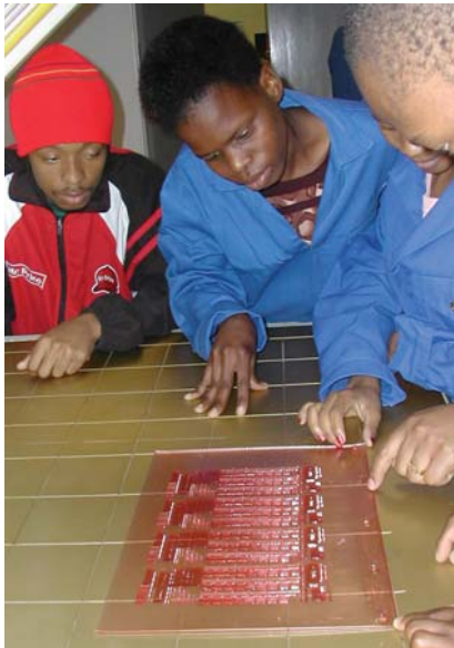
Students examining the quality of a completed Photopolymer plate
